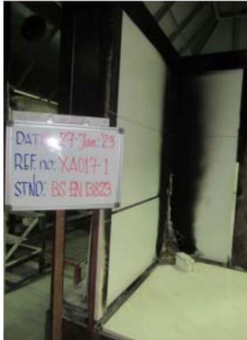
After Fire Test
