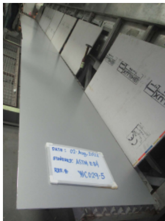
Photo 2: Specimen before the test. (Fire Side)
